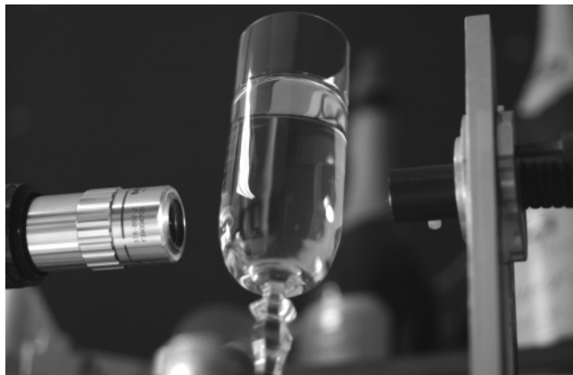
Figure 3. Photographic detail of the workbench used to observe bubble nucleation sites in close-up.
